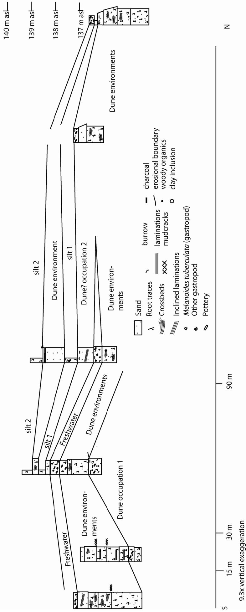
Figure 3. Fence diagram of geologic sections GS001-GS006. Inset shows the portion of Figure 1 in question, with a yellow line indicating the line of section. Sections hang from the upper left corner, which has been set using elevations obtained via total station in the field. Lateral thickness of units indicates grain size, with coarser sands as wider boxes. While details may not be visible, descriptions indicate current environmental interpretations for each unit or set of units.
