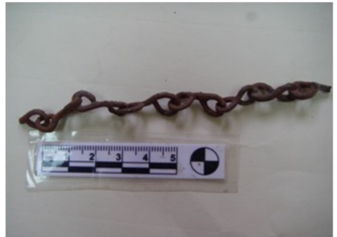
The stages of work of cleaning, separating, and rejoining the pieces of the links in the chain.
