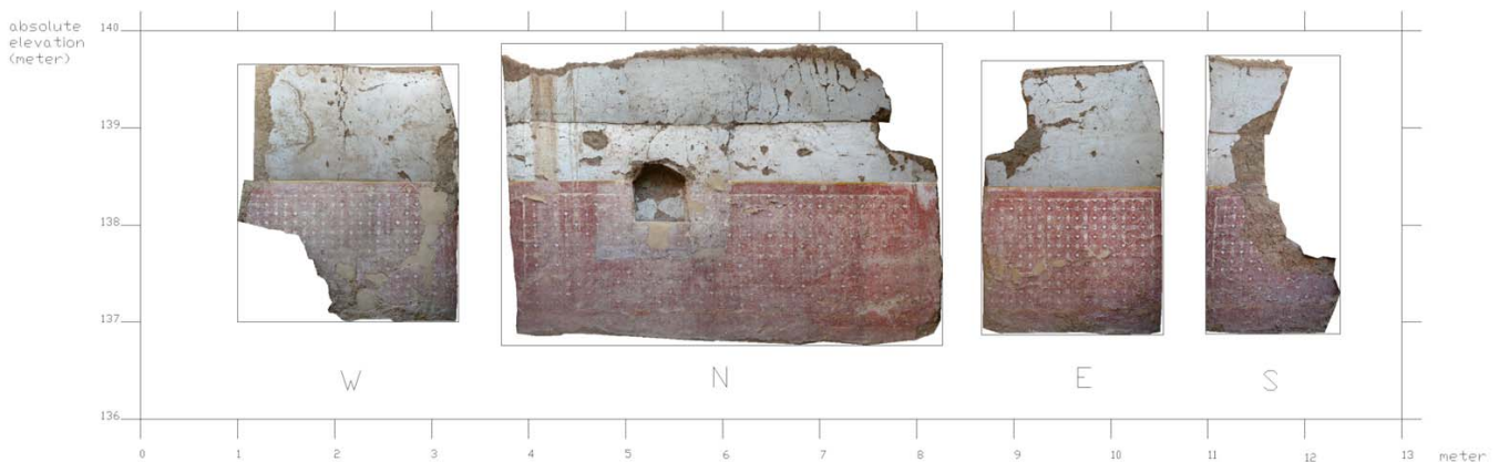
Sample photogrammetric elevations of Room 14
