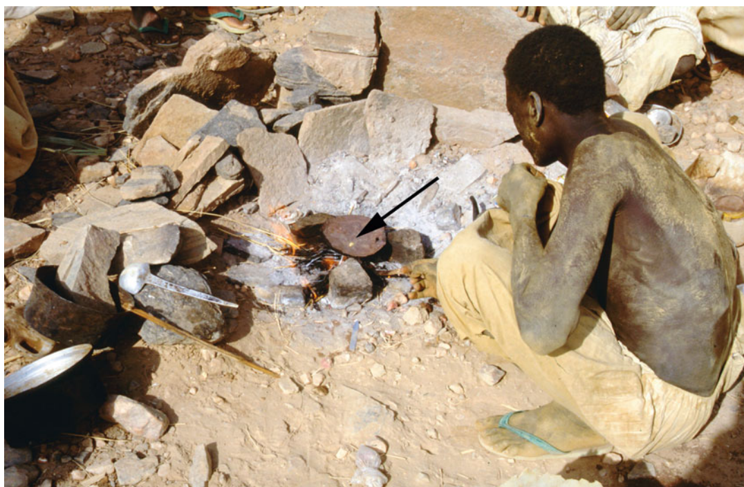
Fig. 6.257 The gold amalgam is heated on a metal sheet in order to evaporate the mercury from pure gold. Umm Sareh, Bayuda
