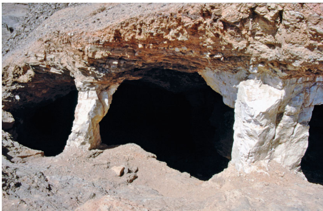
Fig. 6.212 Top row of mouth openings along the heavy quartz vein at Duweishat (shaft 1). Quartz pillars have been left standing to prevent the markedly sheared rock ceiling from caving in
