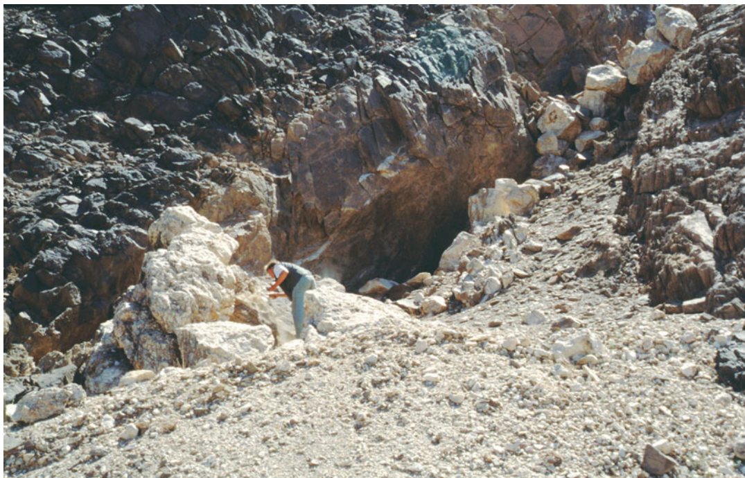
Fig. 6.117 Apparently, only partly productive quartz vein at Khor Nesari 3. The barren (white quartz) areas had therefore been disregarded
