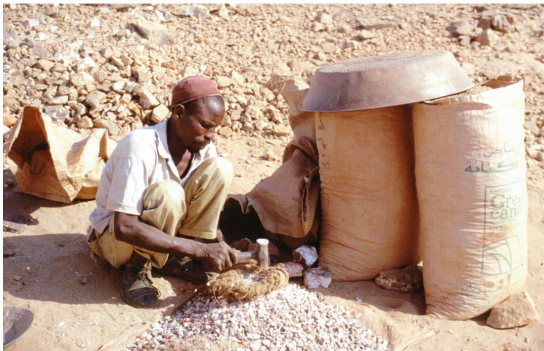
Fig. 6.253 Crushing-down quartz chunks to pea-size before further processing to powder in a diesel-powered ore mill. Hirtawi/Bayuda
