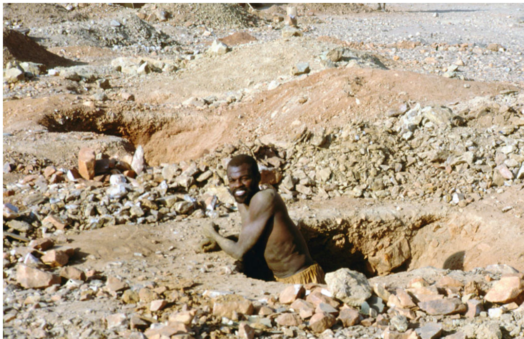
Fig. 6.252 Auriferous quartz chunks are being extracted from wadi sediments in pit holes. El-Higagiya, Bayuda
