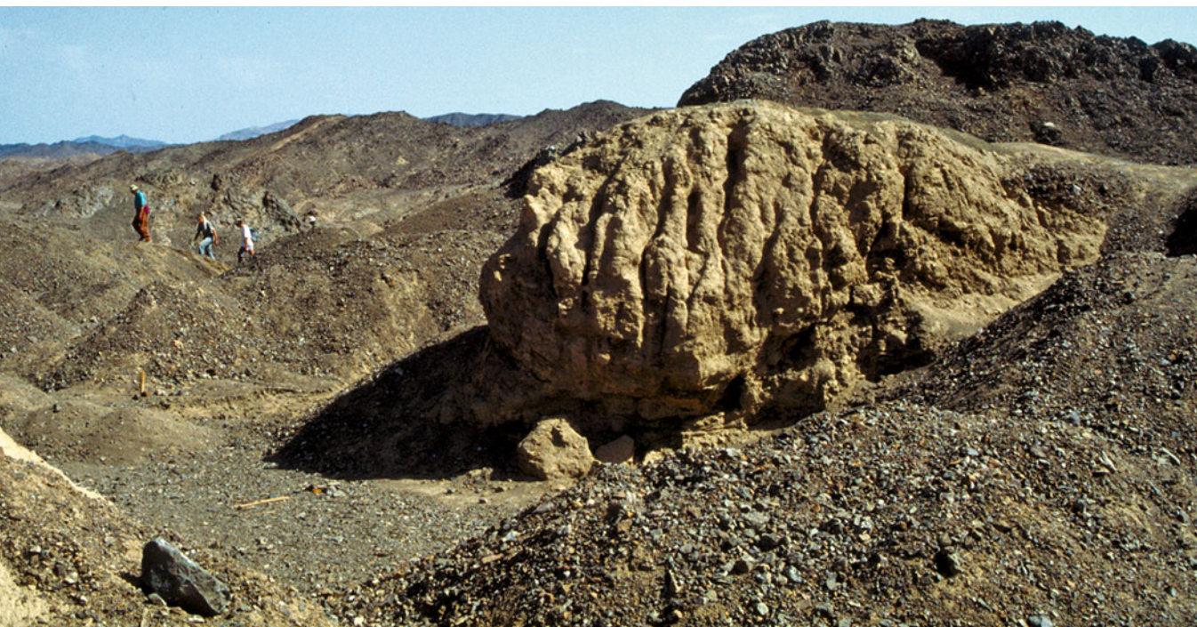
Fig. 1.10 Tailing consisting of processed sand residues. El-Sid mining district, Egypt
