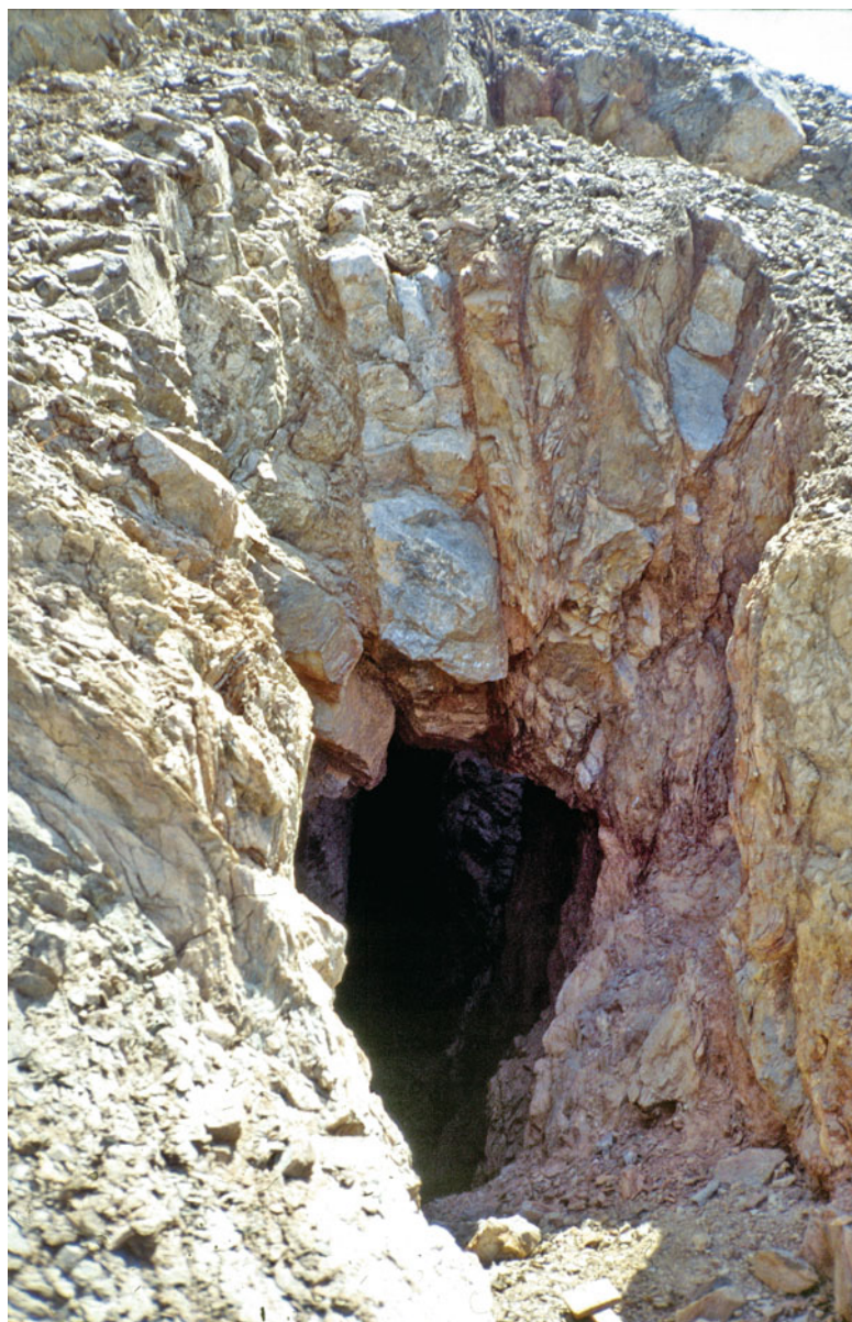
Fig. 5.204 Adit at Umm Ud. Two inclined quartz veins are clearly distinguished. As both proved unproductive at this level, they were mined at deeper depths
