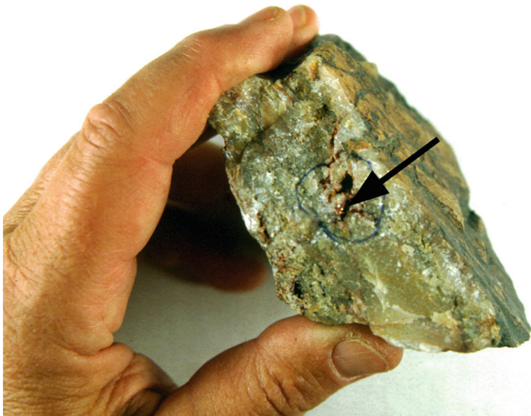
Fig. 6.27 Tiny gold particle ( arrow ) in an originally pyrite-rich cavity of a quartz ore chunk from Tibiri
