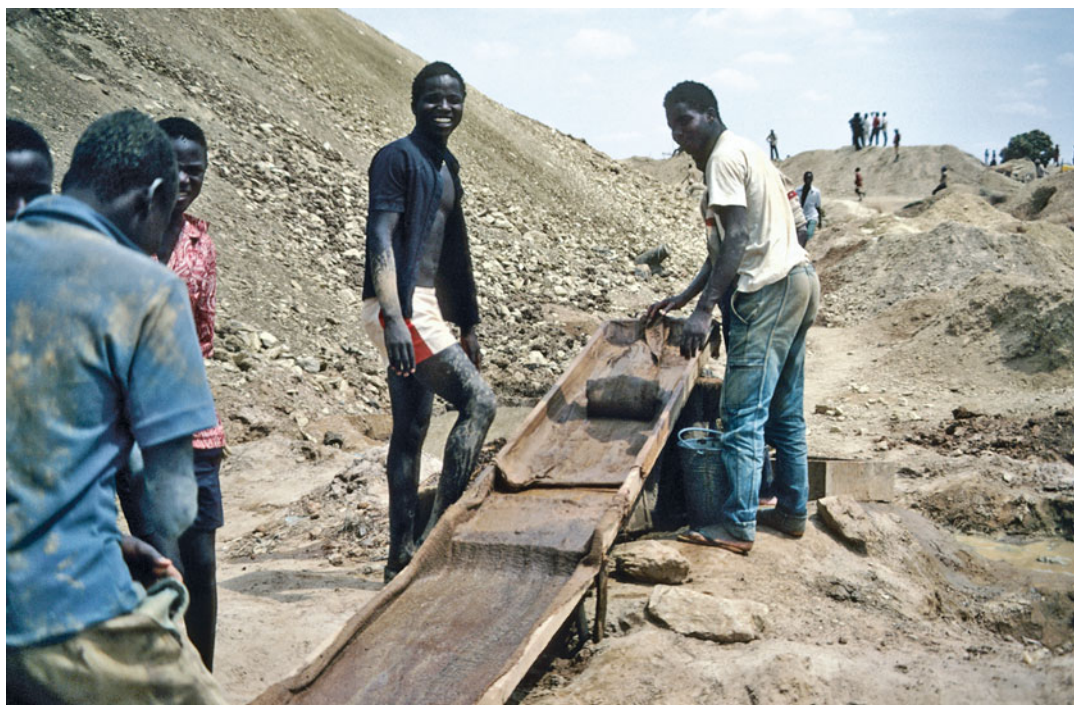
Fig. 1.18 Gold concentrating on a wooden washing frame covered with jute bags to recover the gold particles, Tanzania, 1991. Basically the same method had been
