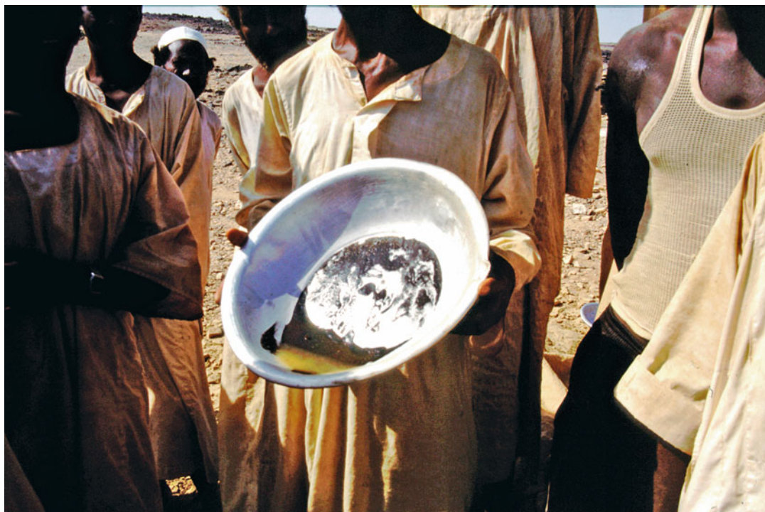
Fig. 6.255 Auriferous, black heavy metal fraction (predominantly magnetite and ilmenite), representing the last stage in the concentration process. Umm Sareh/Bayuda
