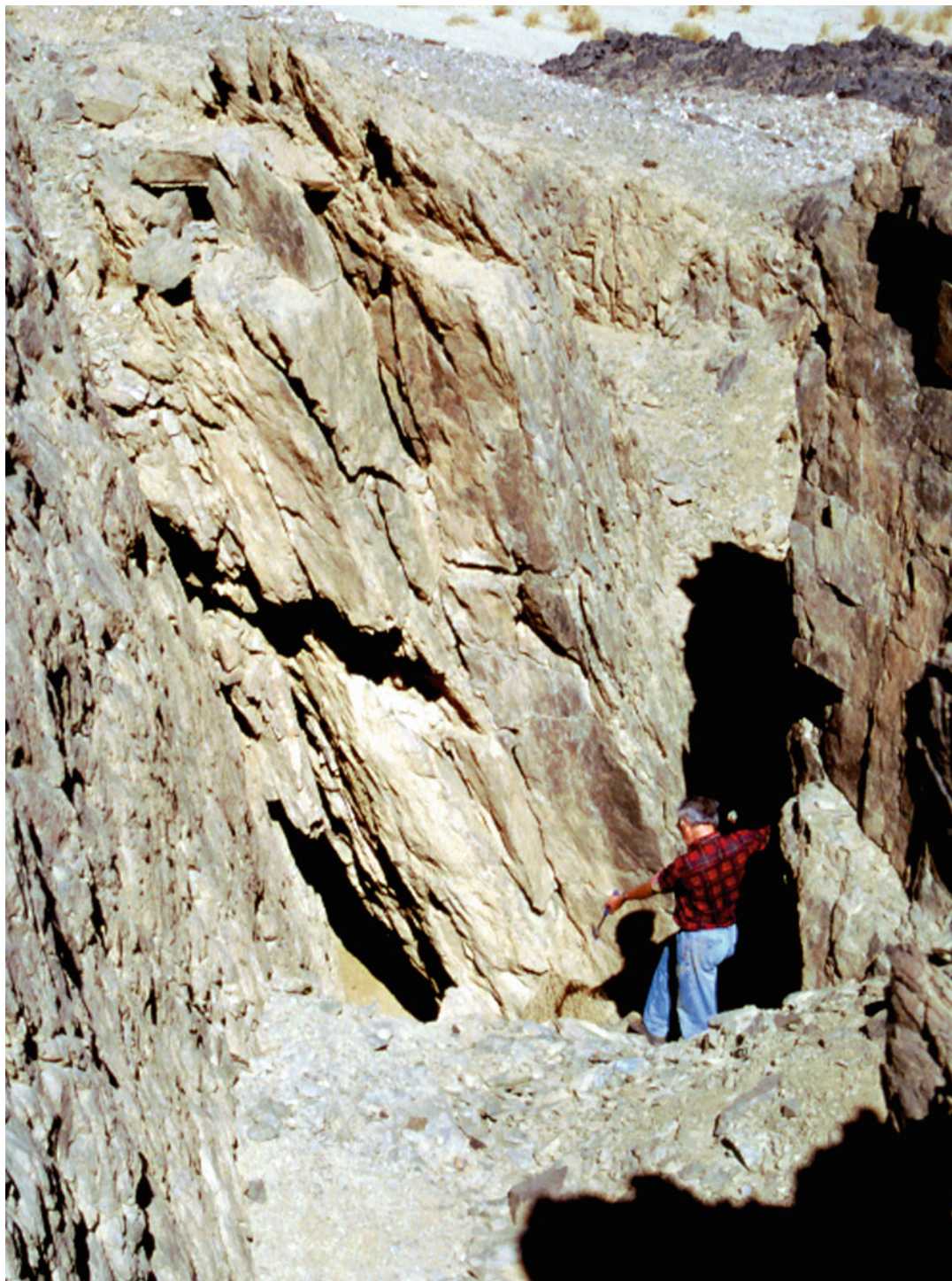
Fig. 6.84 Adit of an exploited, auriferous quartz vein oriented parallel to the foliation at Eikwan 3
