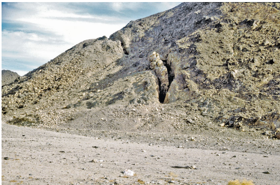
Fig. 5.105 Deep trench pit at Daghabag I. The barren central quartz generation was left behind
