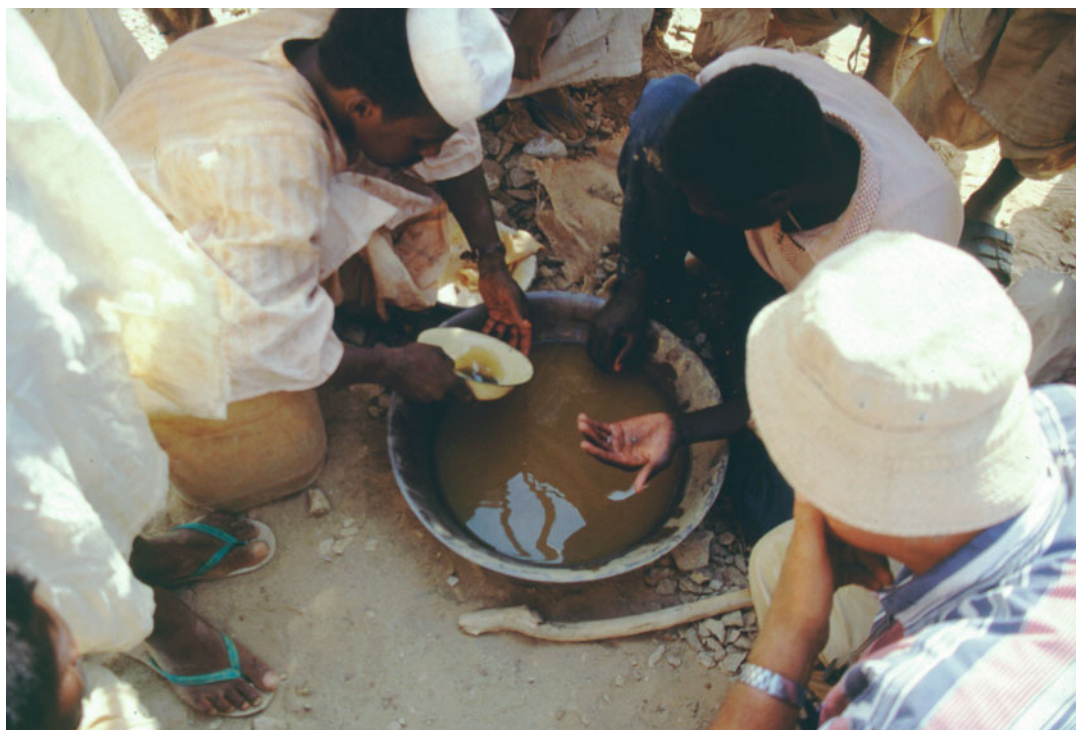
Fig. 6.256 The heavy metals are amalgamised with mercury. Umm Sareh, Bayuda
