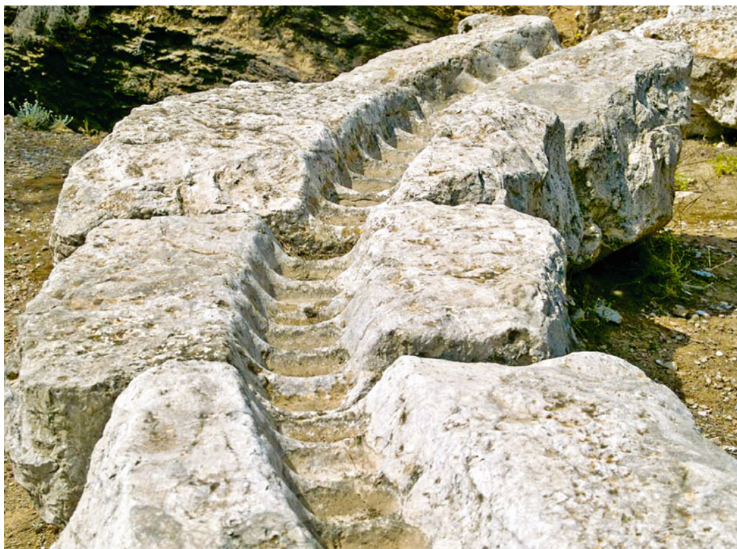
Fig. 5.184 Detail of a “lavérie hélicoïdale” from Laurion/Attica with depressions in the continuous notch for deposition of heavy mineral concentrates (Photo credit: H. Lausch)
