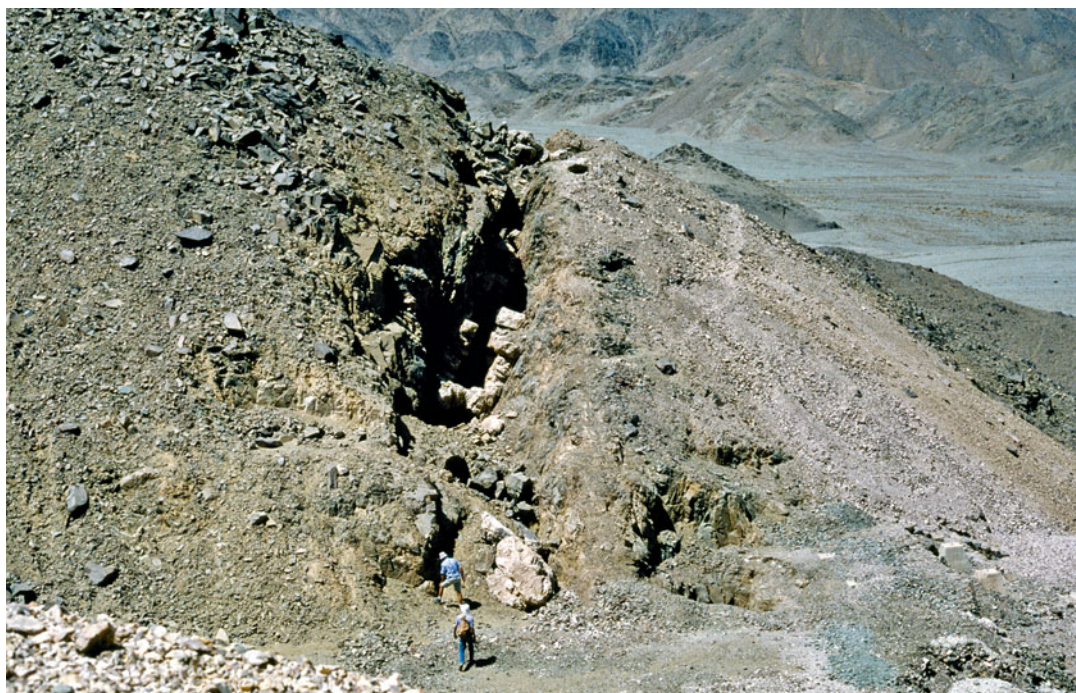
Fig. 5.34 Semna, mined quartz vein showing light-coloured, barren quartzes from an earlier quartz generation. Only its auriferous, central part has been removed
